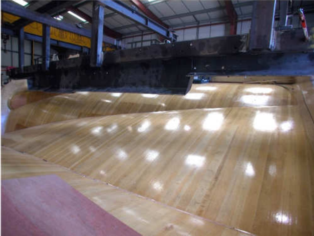
Jelutong engineering pattern - The finished article
